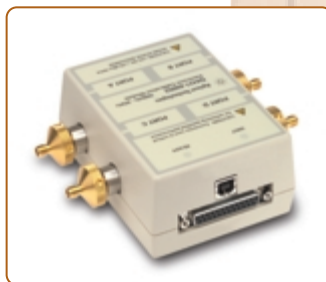
Four-port RF ECal with four 3.5 mm connectors
