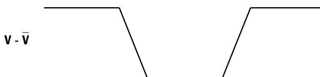
Figure 9. For a differential signal, V - \bar{V} must be \geq 200 mV
