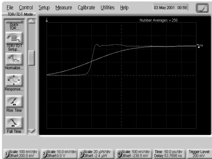
Figure 10. Standard waveform with discontinuities and fast risetime, normalized waveform with a slower default risetime.
