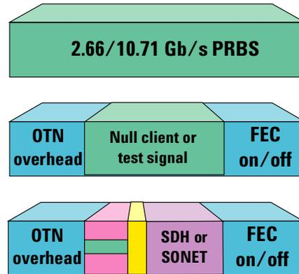
In unframed mode, the instrument tests using a prbs at either 2.66 or 10.71 Gb/s.
