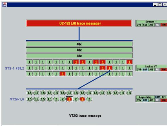
Error and alarm status clearly presented for each detected STS/AU channel, and for all VT/TU channels in a selected STS/AU.
