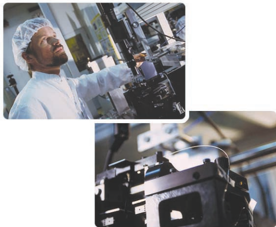
Alcatel's Mr. Koppenborg observes AWG alignment, which requires precise management and highly accurate test equipment. (Photography taken by bild.quelle-Stgt, Tom Pingel)
