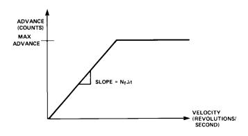
Figure 11. Phase Advance vs. Motor Velocity.
