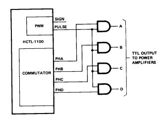
Figure 9. PWM Interface to Brushless DC Motors.
