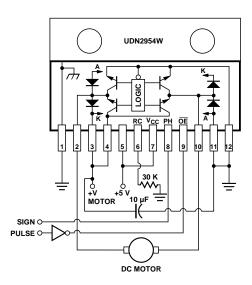
Figure 17. H-Bridge Amplifier Interface.
