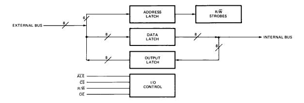
Figure 15. I/O Port Block Diagram.
