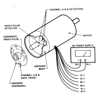
Figure 8. Codewheel Index Pulse Alignment.
