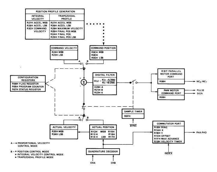
Figure 3. Register Block Diagram.
