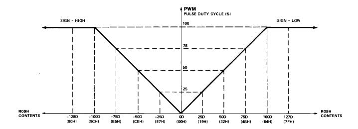
Figure 5. PWM Port Output.
