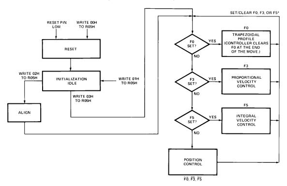
Figure 2. Operating Mode Flowchart.
