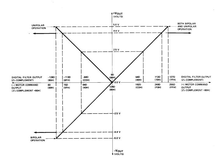
Figure 4. Motor Command Port Output.
