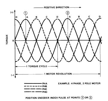
Figure 7. Index Pulse Alignment to Motor Torque Curves.
