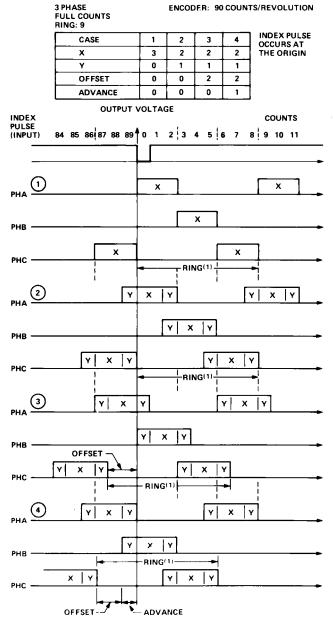
Figure 10. Commutator Configuration.
