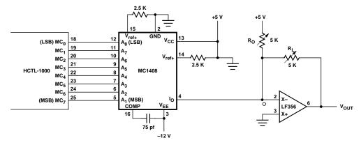
Figure 16. Linear Amplifier Interface.
