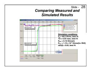
We use the resistive losses from the field solver and optimize the values of TD and the dissipation factor to give the best agreement with the TDR/TDT measured data.
