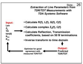
The extraction software that allows the prediction of TDR and TDT measurements, was developed by TDA Systems. The basic algorithm is to select values of the basic parameters that describe a lossy line: the length, the characteristic impedance, the time delay, the DC resistance, the term proportional to root frequency and the dissipation factor.
