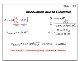
We have a way of describing each of the loss terms, the resistance and conductance per length of the lossy line. These two terms factor into the attenuation of the line.
