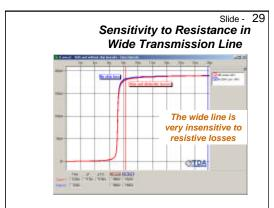
In this particular example, we designed the test vehicle to be insensitive to the resistive loss so we would be more sensitive to dielectric loss. We can confirm this by comparing the predicted response with no resistance used in the input and with the values suggested by the field solver.
