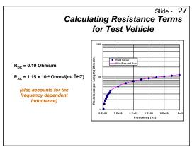
The resistance terms for the meander test pattern can be extracted with a 2D field solvers, such as the Ansoft Maxwell 2D Extractor.
