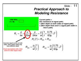
This simple model illustrates the features of the resistance. There is a DC term that is due to the geometrical cross section, and there is an AC term that is proportional to the square root of frequency. Both of these terms can be calculated directly, given the resistivity and the geometry of the transmission line.
