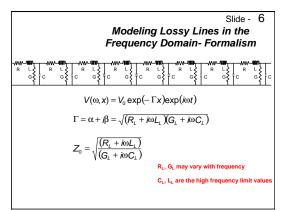
To model attenuation in a transmission line, we need to add the lossy elements of the series resistance per length and the shunt conductance per length to the typical lossless equivalent circuit model for a transmission line. This model is shown in this figure. The conductance term is really a resistor that represents the AC loss of the dielectric.
