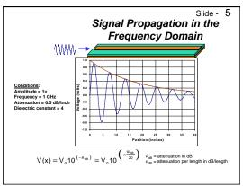
Analyzing the lossy effects in transmission lines is much easier in the frequency domain. Of, course, in the frequency domain, the only signals that exist are sine waves.
