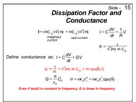
The resistive current through a capacitor can be represented by a resistor that is frequency dependent. Because this resistor is shunting the capacitor, it is often referred to not as R, but as a conductance, G. The value of the conductance is related to the imaginary part of the dielectric constant or the dissipation factor.
