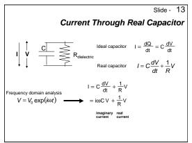
The second loss term is the dielectric loss. The easiest way to think about the dielectric loss is to model a real capacitor filled with real dielectric as an ideal lossless capacitor and a resistor that gives rise to resistive loss of energy.
