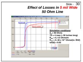
In typical back plane or large motherboard applications, the line width might be on the order of 5 mils. In this case, the resistive losses play a dominate role.
