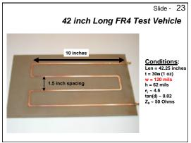
The DUT is a custom manufactured serpentine microstrip on an 062 mil thick FR4 substrate. In
