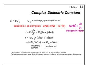
To take advantage of the properties of complex numbers, this real and imaginary current through a real capacitor can be modeled by changing the nature of what is commonly referred to as the dielectric constant.
