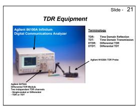
To perform the measurements, an Agilent 86100A Infinium Digital Communications Analyzer mainframe was used. An Agilent 54754A differential TDR plug in was used to take the TDR and TDT data.
