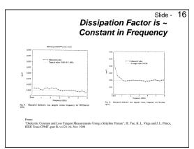
Most dielectric materials have a dissipation factor that is roughly constant with frequency. In this example, a Duroid® material and an FR4 sample were measured and the dissipation factors are seen to be constant above about 800 MHz.
