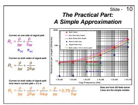
The resistance per length can be calculated from the cross sectional area. We assume a simple behavior that the resistance is a DC term that is just related to the geometrical cross section and an additional term that is the cross section corresponding to the skin depth thickness.
