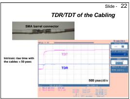
The first step is evaluating the performance of the cabling that will hook up to the device under test (DUT).
