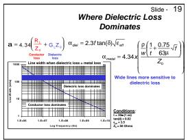
From this simple model, we can evaluate at what line width will dielectric losses equal resistive losses, for a 50 Ohm line. At any frequency, there will be a line width where these two terms are equal.
