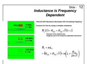
For the same reason that resistance is frequency dependent, the inductance will be. The current distribution changes and the internal self inductance of the current loop will decrease at higher frequency.
