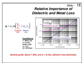
Based on these simple models for the resistance and dielectric loss, we can approximate the attenuation from each of the sources.
