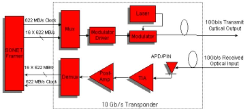
**10 Gb/s Fiber Optic Transponder Block Diagram**
