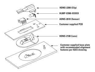
Figure 2. Exploded view drawing of optical mouse components.
