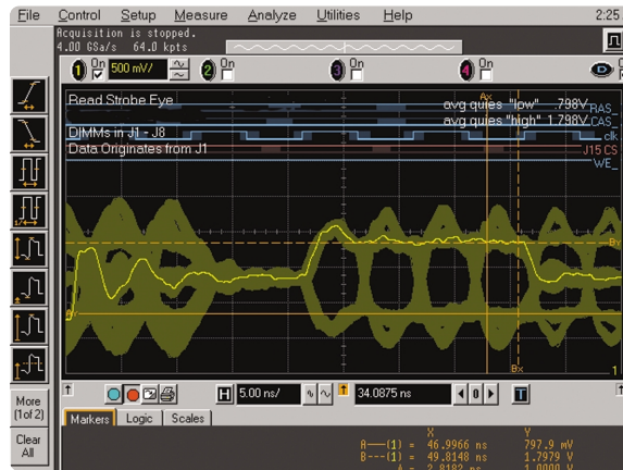
Figure 3. A view of data bit D0 with analog scope channel 1 exclusively for data "reads" (bottom) by setting a trigger on the five control lines (top)
