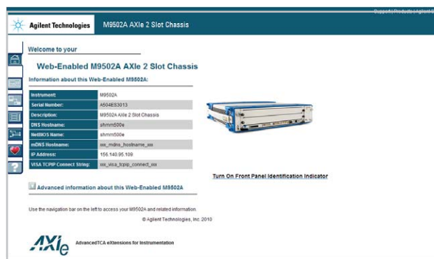
Figure 1. AXIe chassis web server
