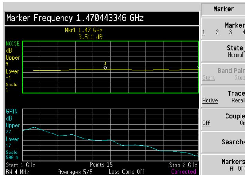
Turn the RPG to place the marker at the point on the trace you want to measure or use the numeric keys to enter the frequency of interest.
