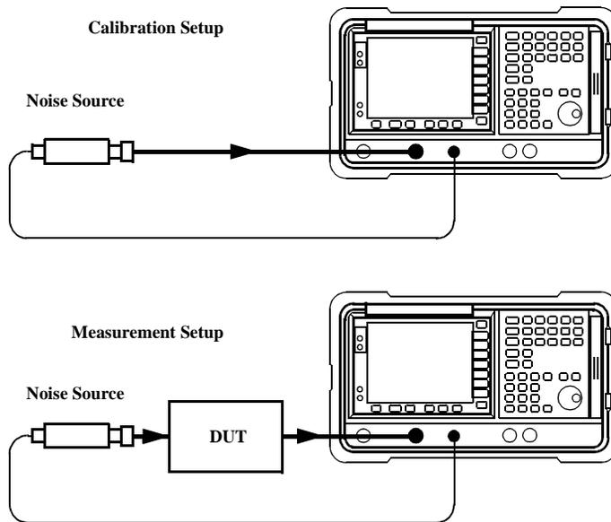
When an uncorrected measurement is performed, the result is the measured Noise Figure of all of the components after the noise source. When the calibration setup is connected and the calibration performed, the NFA measures its own noise figure. When a corrected measurement is performed, the contribution of the calibration setup is removed from the uncorrected result, giving a corrected measurement of the DUT only.
