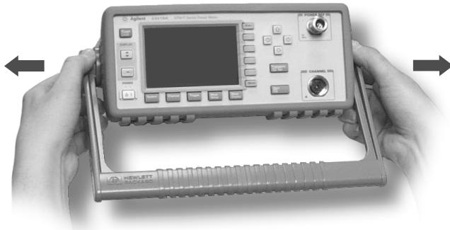
If you want to remove the handle, refer to Rack Mounting the Power Meter on page 30.
