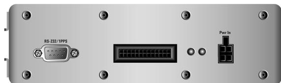
**Figure 23** Serial port on GPS/DR unit
