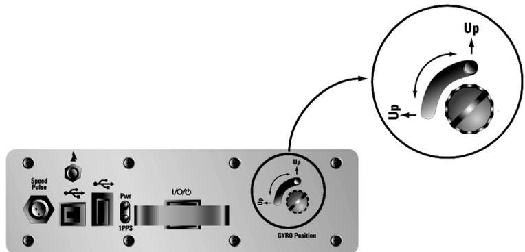
**Figure 24** Setting the Gyro pin. If the unit is set on its right side, the pin is set at the alternate position.
