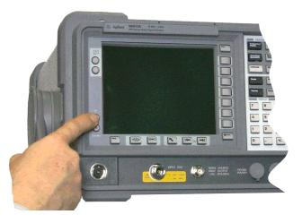
**Welcome screen** Upon power-up, a welcome screen appears and when the Noise Figure Analyzer is ready for use, the welcome screen clears from the display.
