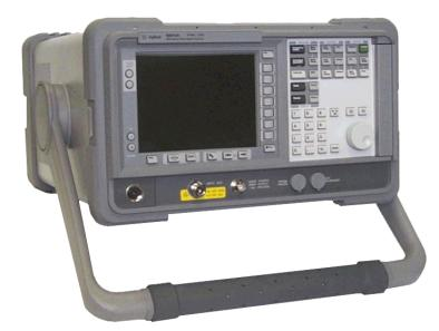
**CAUTION** When installing the product in a cabinet, the convection into and out of the product must not be restricted. The ambient temperature (outside the cabinet) must be less than the maximum operating temperature of the product by 4 °C for every 100 watts dissipated in the cabinet. If the total power dissipated in the cabinet is greater than 800 watts, then forced convection must be used.
