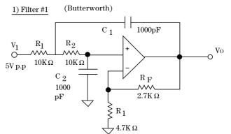
Important - Monitor the input and check/re-adjust to proper 5V p-p at each frequency.
