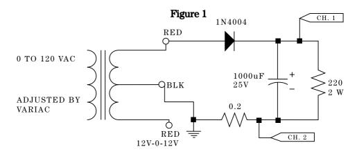
To observe the steady-state DC output voltage with its ripple, Channel 1 is connected to the top of the load resistor and the oscilloscope is used in a conventional repetitively-triggered mode. The automatic measurement capabilities of the oscilloscope can be used to quantify the peak, average and RMS values of an unfiltered rectifier.
