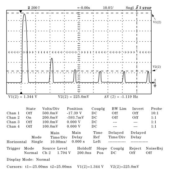
Figure 2 - Diode Current vs. Time, Showing Large First-Cycle In-rush Current
