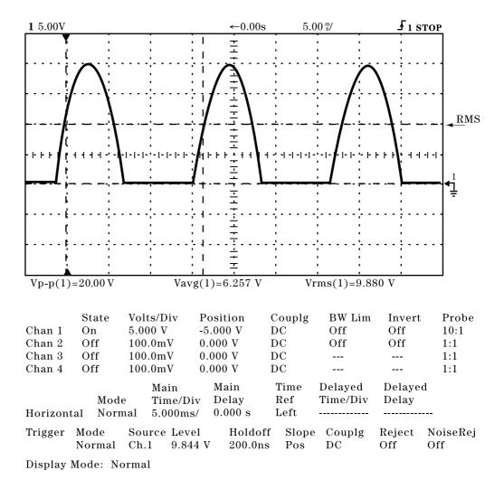
Figure 5 - Unfiltered Rectifier Output Voltage, With Automatic Voltage Measurements
