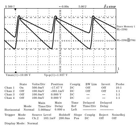
Figure 4 - Filtered Rectifier Output Voltage For Two Different Load Resistors (Using Trace Memory)
