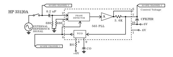
The PLL is free-running until the SPST switch is closed. The PLL then goes from its free-running condition to its locked condition in a process known as **acquisition**.
