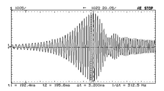
The cursors measured the frequency at the peak of the waveform, and voila... the same resonance that we saw in the FFT example. For a little more resolution, I spread the waveform some more, and found the resonance to be at about 333 Hz:
