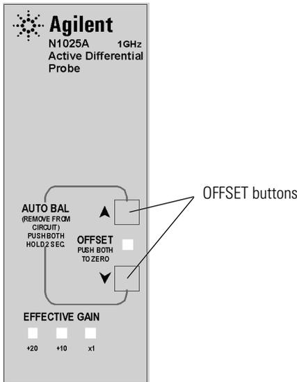
Upon successful completion of the AutoBalance cycle, all three of the **EFFECTIVE GAIN** indicators will be briefly illuminated. If an input signal is present during auto balance and the routine fails, the **EFFECTIVE GAIN** indicators will not illuminate. The probe will then revert to the offset values resulting from the last successful completion of the AutoBalance cycle. In many situations, this will be adequate to make routine measurements.
