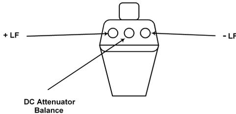
The attenuator's plastic covers may be removed. Take care not to damage the probe attenuator pins.
