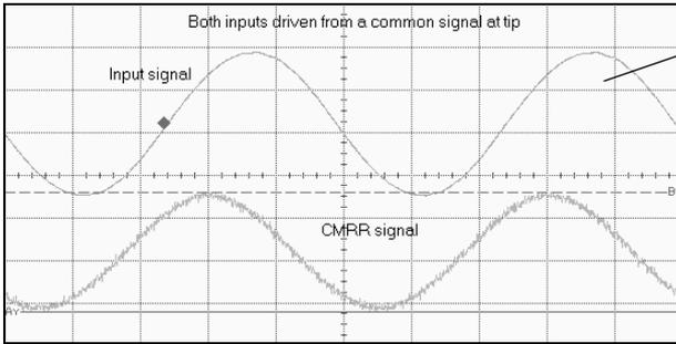
Both inputs derived from a common signal at probe tip.
