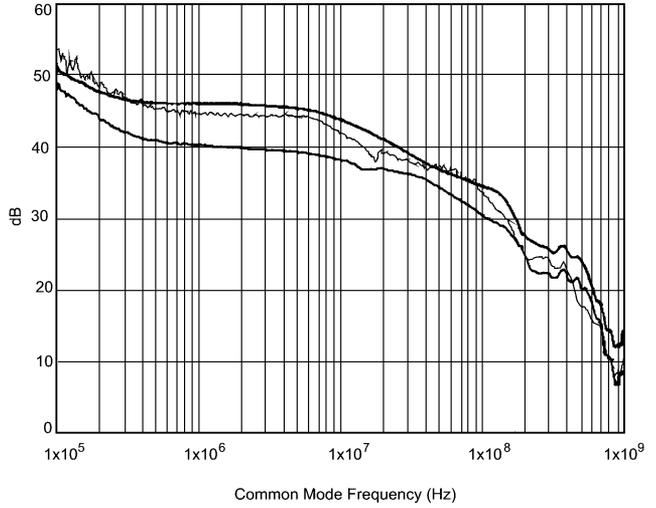
**Typical CMRR versus Frequency (Hz)**
