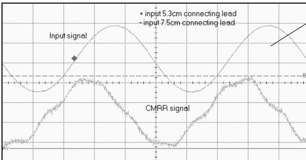
Probe coupling leads of different length. Positive input 5.3 cm. Negative input 7.5 cm.
