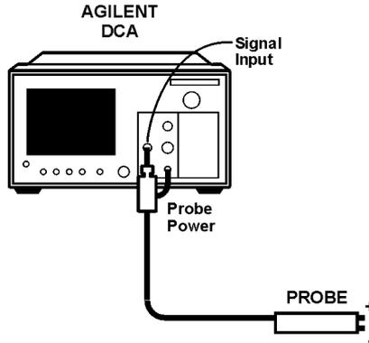
**Figure 5-1. AutoBalancing the probe.**
