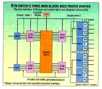
chips or boards within communication designs. Boards or chips from different design groups or vendors that follow this standard can be easily integrated. Today, practically all available commercial ATM chips or modules (e.g., Line Interfaces) claim to be Utopia compatible.
