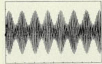
Figure 5A. An amplitude-modulated carrier in the time domain.
