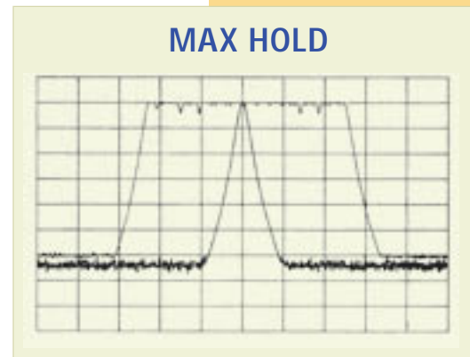
Figure 31. The MAX-HOLD mode is used to measure the peak frequency deviation.
