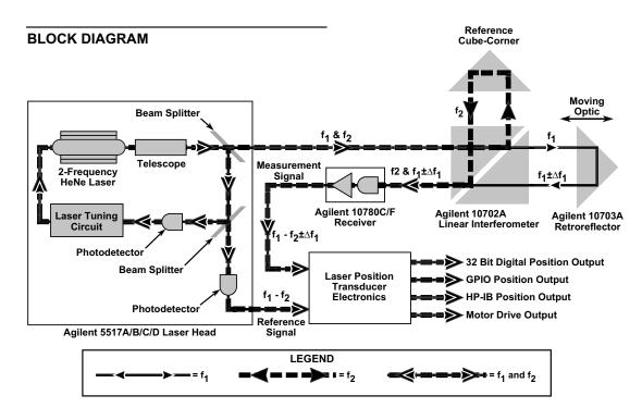
Figure 14-1. Typical (older) Agilent Laser Position Transducer block diagram
