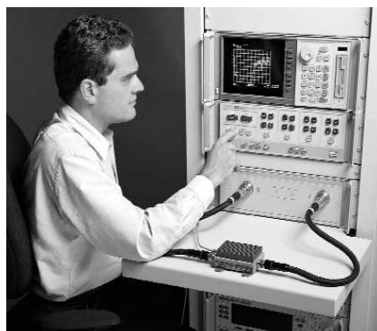
The Agilent 85108 A/L offer pulsed-RF measurements in frequency and time domain.
