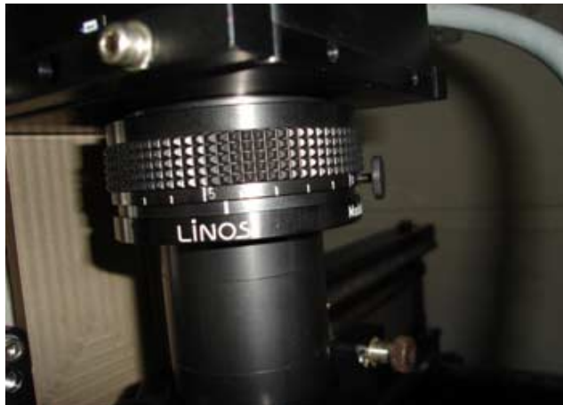
Figure 7-1 Focus ring on the camera lens
