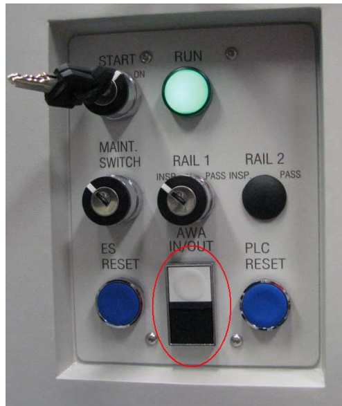
Figure 5-2 AWA IN/OUT buttons on the switch plate
