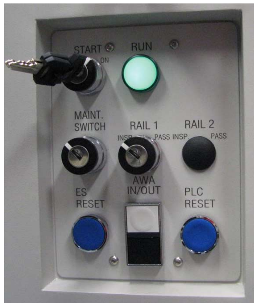
Figure 4-1 Controls on the switch plate at the front of the machine
