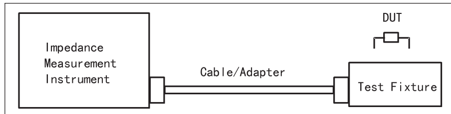
System configuration for impedance measurement
