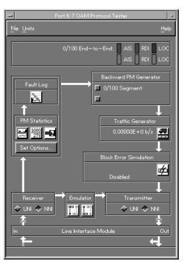
The E6270A OAM Protocol Tester turns the industry-standard Agilent Broadband Series Test System (BSTS) into an OAM test tool with powerful traffic generation and real-time QoS measurement capability.
