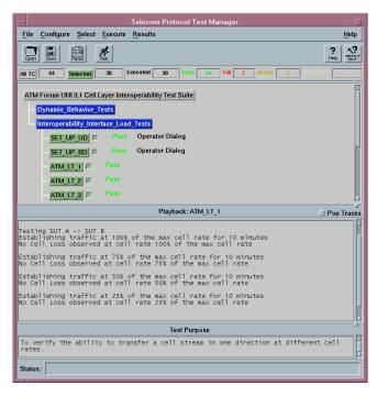
The Test Manager test execution environment that runs on the Agilent broadband tester
