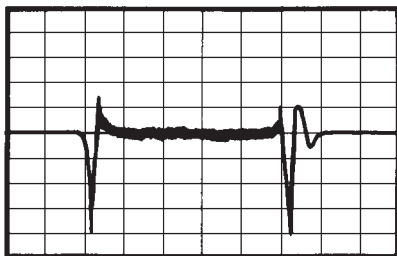
Figure 21. Phase transients at output of phase detector as observed on an oscilloscope connected to the AUX monitor port
