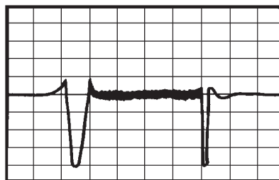
Figure 22. Phase transients with saturation as observed on an oscilloscope connected to AUX monitor port
