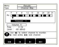
At-a-glance display of active timeslots, frequency and level measurements combined with the ability to listen to timeslots.
