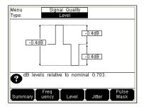
Easily identify any frequency, level, pulse shape or jitter problems.
