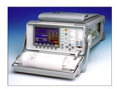
The OmniBER 718 analyzer is a rugged, portable one-box solution for installation, maintenance and manufacturing of SDH/SONET networks and network elements. It provides full PDH/T-carrier and SDH/SONET capability up to 2.5 Gb/s, including STM-16c/OC-48c payloads and jitter.
