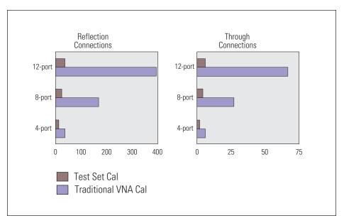
Test Set Cal reduces the number of connections required to calibrate all possible measurement paths.
