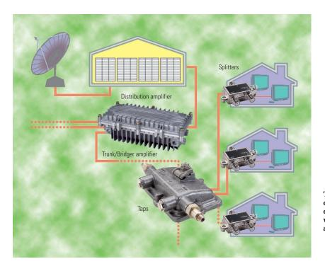
This schematic of a cable-TV distribution system shows some of the devices that can be easily measured with an 87075C multiport test set and an 8712ET/ES network analyzer.
