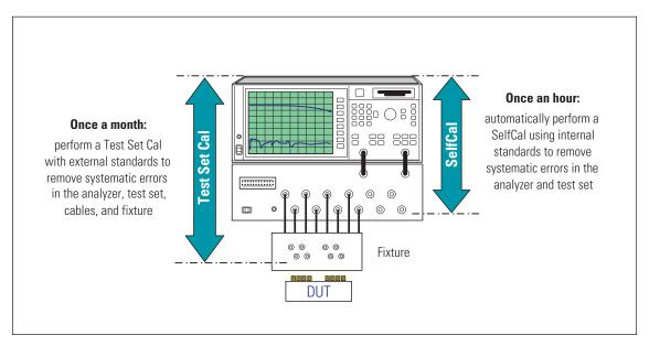
Test Set Cal and SelfCal can give you up to three extra days each month (per test station) for increased production.
