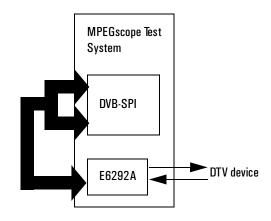
The SMPTE 310M internal interface is connected to the DVB-SPI through an external cable.
