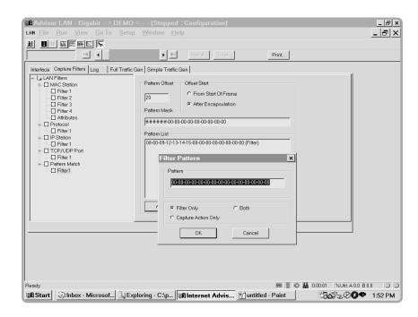
All filters work in node mode as well as pass-through mode on both channels. Station filters may be defined as "to" and or "from":
