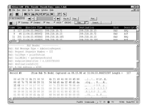
The Ethernet Advisor provides 7-layer decodes of all major protocols, including 802.1p, 802.1Q and 802.3x. Protocol decodes have a built-in protocol follower that will flag errors as they occur. A convenient "Go to next error" feature allows you to advance to the next errored frame in the capture buffer.
