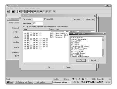
It provides intelligent packet and capture buffer file editing for full seven-layer customization of data to be transmitted. While you specify frame rate, burst count, or percent utilization, the software automatically calculates inter-packet gaps for various traffic loads, calculates the checksum and generates a CRC.
