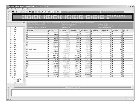
This raw data is correlated and displayed on an easy to understand Graphical User Interface. Five separate views organize the switches data, allowing the user to concentrate on the data of interest, presenting pertinent statistical and graphical information needed to assess the health of the data being processed by the switch. Select which port to monitor via the "explorer" navigation menu or "clicking" on the port of interest.
