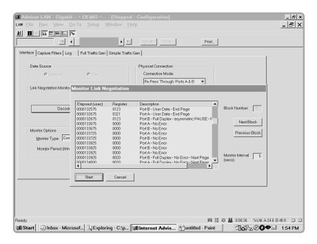
While the link negotiation monitor is running, no other measurements are available.
