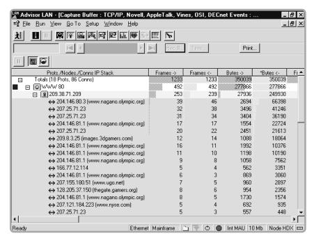
Right click on any column heading and select "Sort by this column" to sort the information for you by the chosen category. Data capture filters may be set while running these measurements, so that only a specific set of nodes is included.
