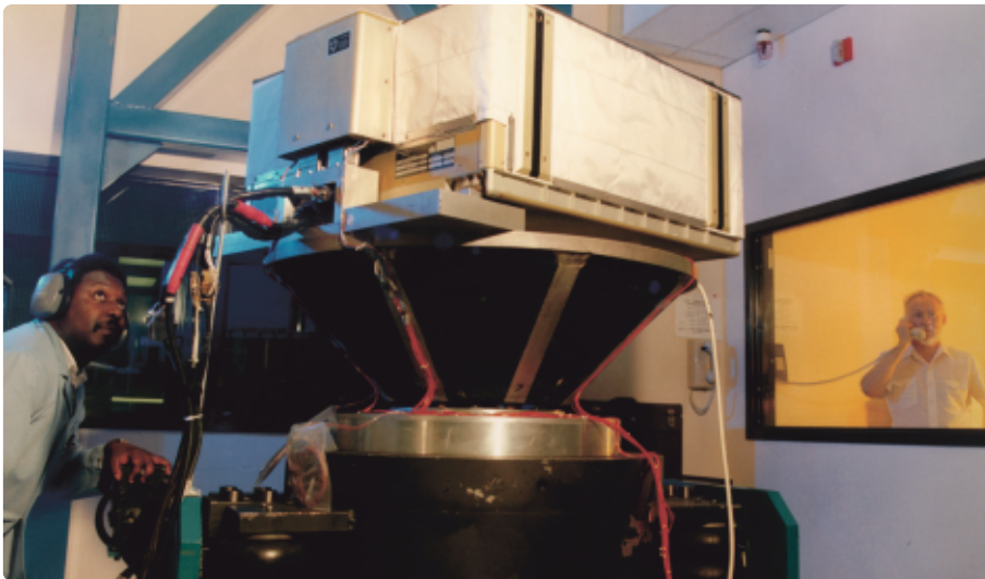
SS/L senior battery technician, Kenny Cox (left), and vibration test conductor, Ed Eckert (right), monitor an International Space Station Battery Orbital Replacement Unit (ORU) during qualification-level vibration testing. The test, which was successfully conducted, ensures that the Battery ORU will sustain the heavy launch loads of the Space Shuttle. Following this test, SS/L successfully completed qualification-level thermal vacuum, thermal cycling, and electrical performance tests.
