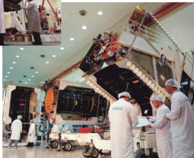
SS/L integration technicians have completed communication panel integration on Sirius FM-01. Sirius FM-02 continues to receive harness routing and lower bus electrical systems testing. Sirius FM-03 was delivered to the assembly floor after completion of propulsion systems integration.
