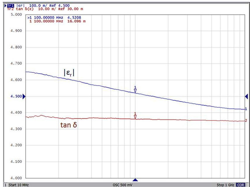
Figure 23. Frequency response of glass epoxy ( \epsilon_r = 4.5 )
