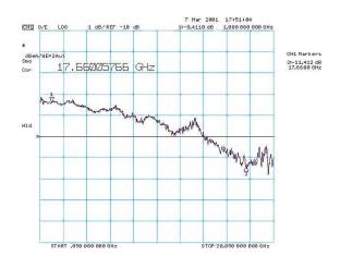
3 dB bandwidth measurements can be easily automated on the 8703B.
