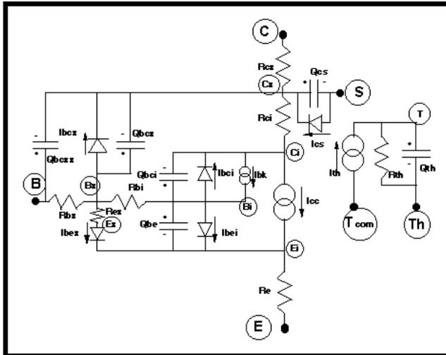
Figure 2-1. Circuit diagram for large signal HBT model
