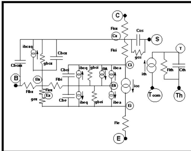
Figure 2-2. Circuit diagram for small signal HBT model
