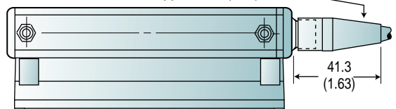
Solenoid Drive Plug and 5 ft. cable supplied, 6.3 (0.25) dia.
