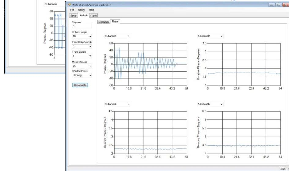
Cross-channel (relative) phase after isolating measurement Intervals
