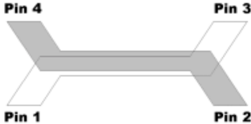
Surface Mount 3dB Coupler Layout
