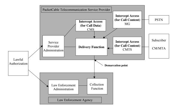
Figure 1 - Electronic Surveillance Model
