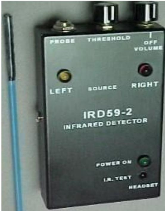
As the probe is passed through the IR beam either the yellow LEFT light emitting diode (LED) or the red RIGHT LED will light. When the IR source is to the left of the unit, the LEFT LED flashes and an internal vibrator pulses on and off. When the IR source is to the right of the unit, the RIGHT LED remains lit and the vibrator runs continuously. The unit detects both continuous wave or modulated beams.
