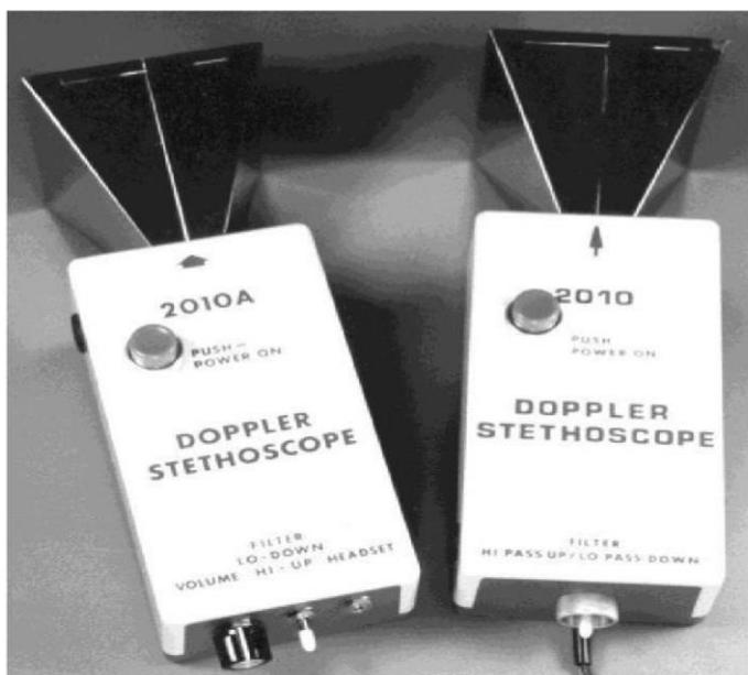
The 2010/2010A Doppler stethoscopes were truly amazing devices. I had accidentally discovered the principle behind the homodyne module (transmitter and receiver combined) while working on my Super Man X-ray which I envisioned being able to see inside packages. With them you could hear timers inside soft sided packages such as cardboard boxes, attache cases, suitcases and even PVC pipes. It also detected radio controlled improvised explosive devices.
