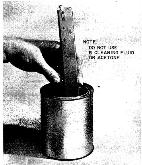
**Fig. 8—Soaking F Connector Presser**
