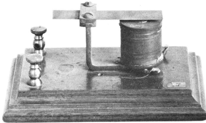
Figure 1-2 Vibrating Reed Receiver
