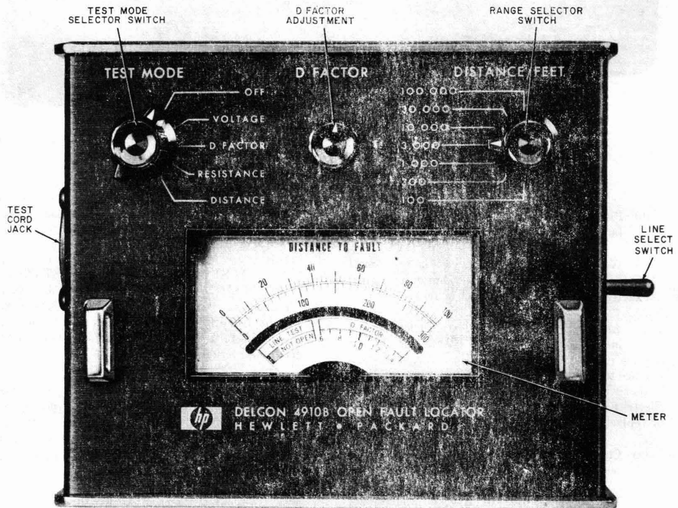
Fig. 4—Meter And Controls On Delcon 4910B
