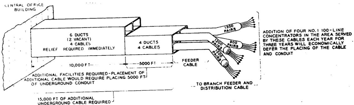
Figure 15-25 - Temporary Use of Concentrators
