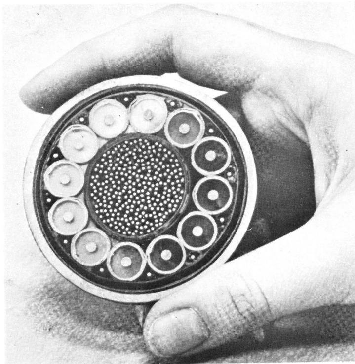
Figure 15-11 - Coaxial Cross-Section
