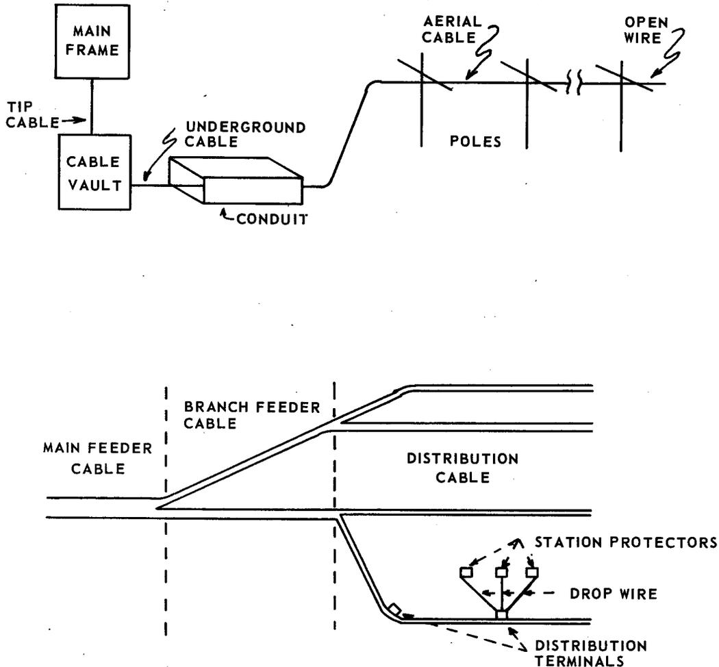
Figure 15-1 - Typical Cable Run -
