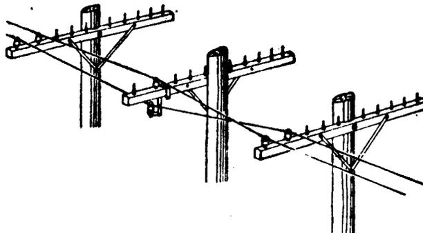
Figure 15-8 - Drop-Bracket Transposition
