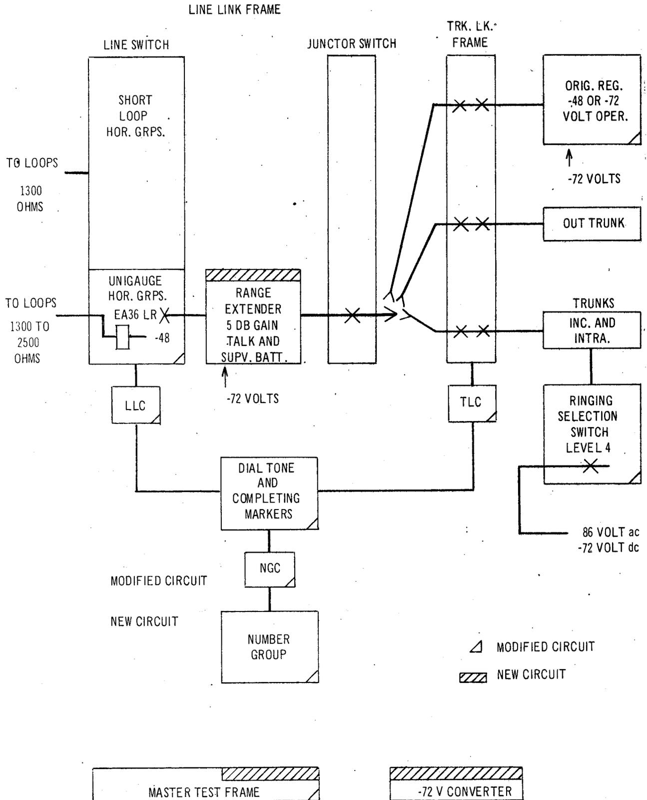
Figure 15-33 - Unigaug No. 5 Crossbar Switching Plan
