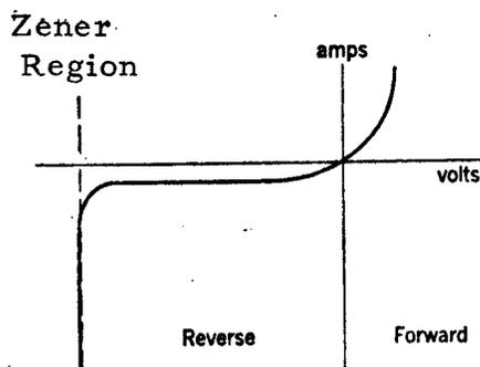
Figure 15-24 - Diode Characteristic
