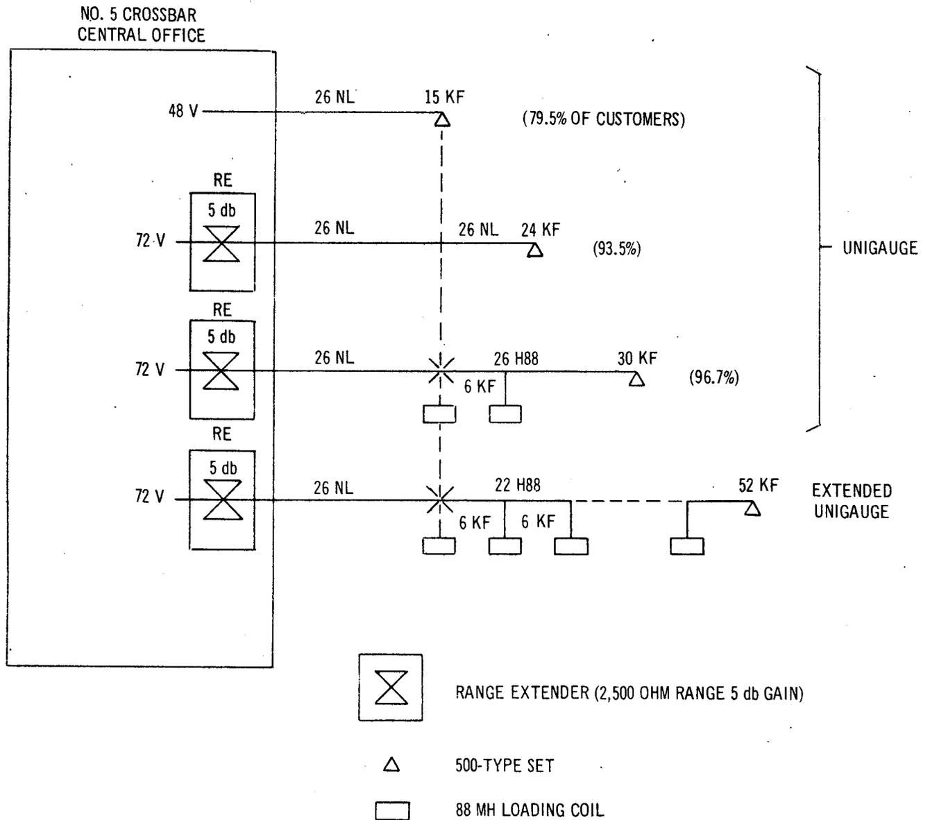
Figure 15-31 - Uniform Gauge Loop Plant Layout
