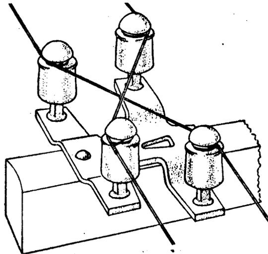
Figure 15-7 - Point-Type Transposition
