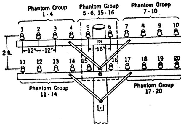
Figure 15-5 - Wire Configuration For Open Wire Line (Side and Phantom Circuits)
