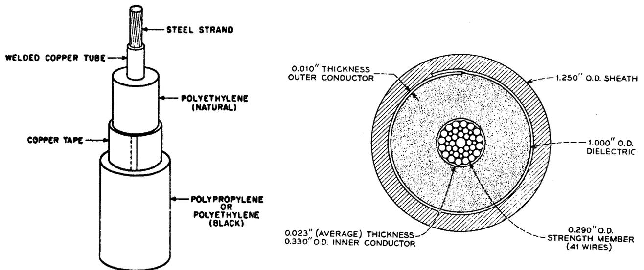
Figure 15-15 - Ocean Cable (Armorless-Lightweight)
