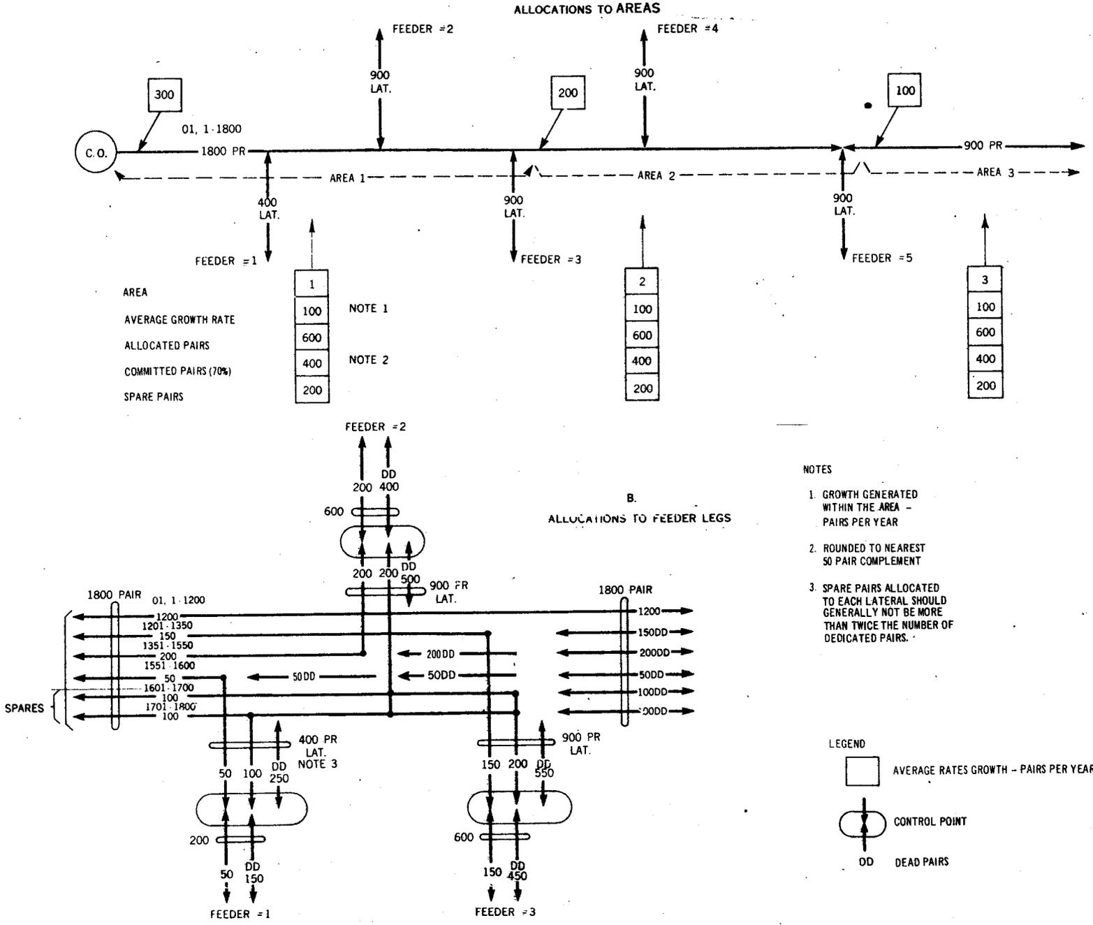
Figure 15-29 - Pair Allocations To Areas and Feeder Legs
