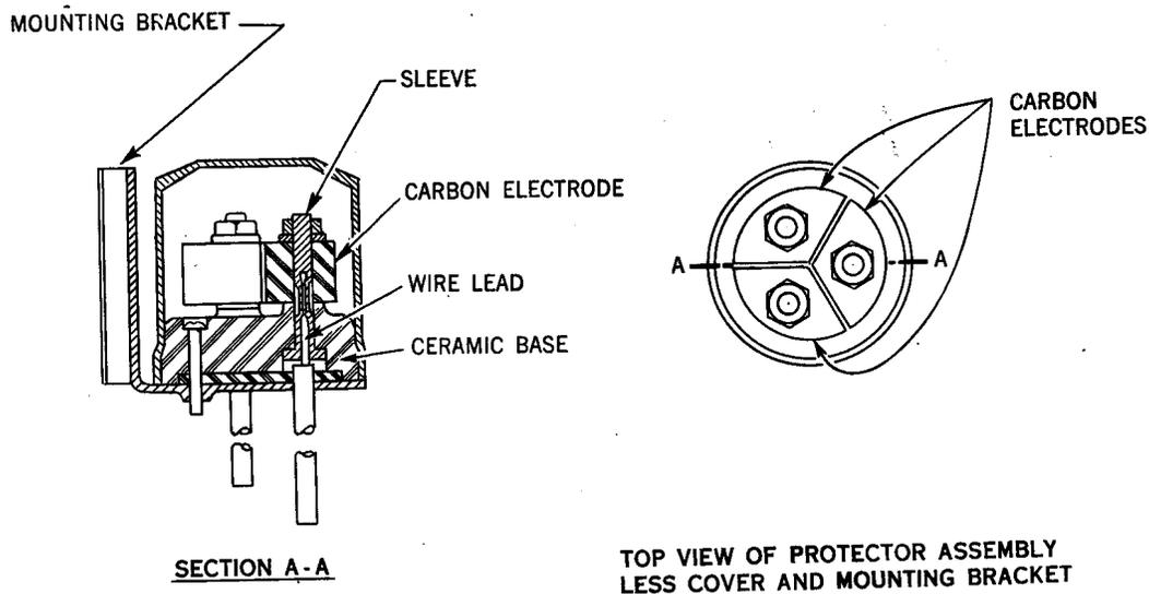
Figure 15-22 - Heavy Duty Protector In Weatherproof Mounting
