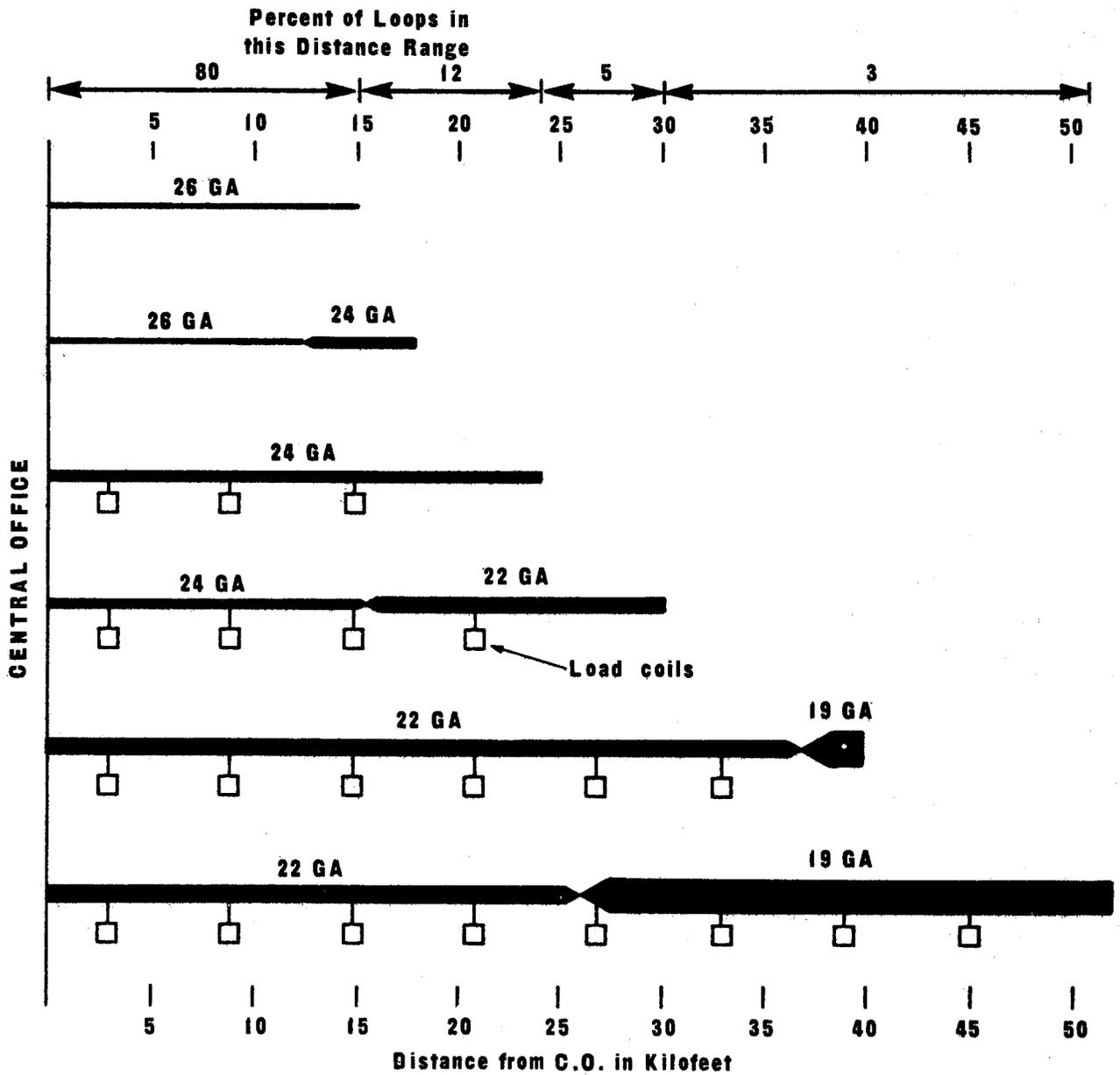
Figure 15-30 - Cable Plant Gauge Composition Resistance Design
