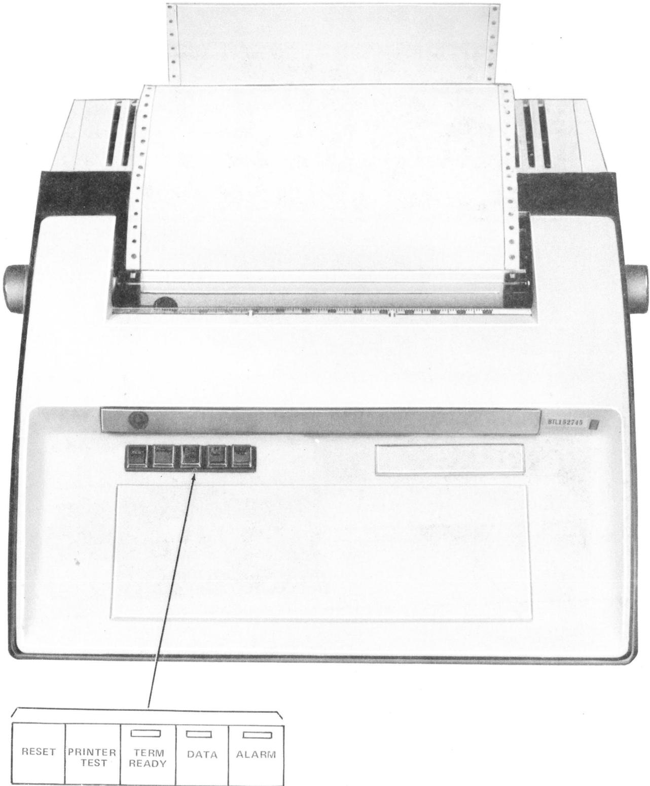
Fig. 4—Receive-Only Printer
