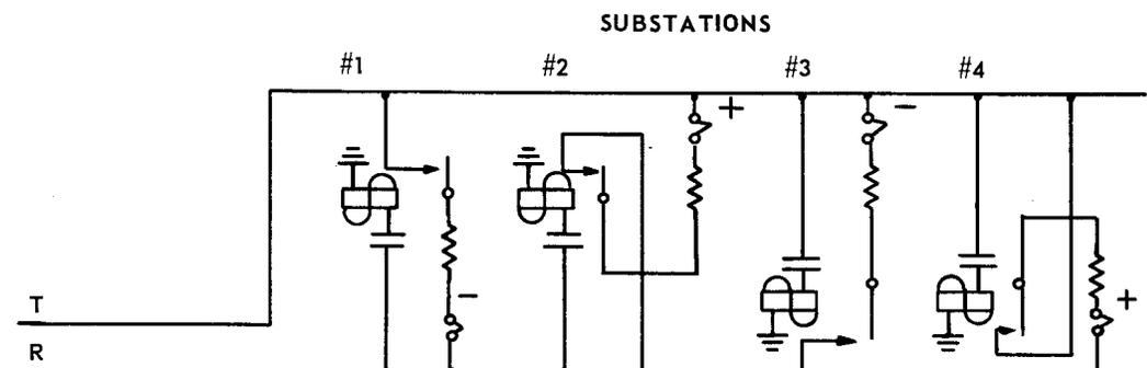
Figure 2-19 Inverted Relay Biased Bell System
