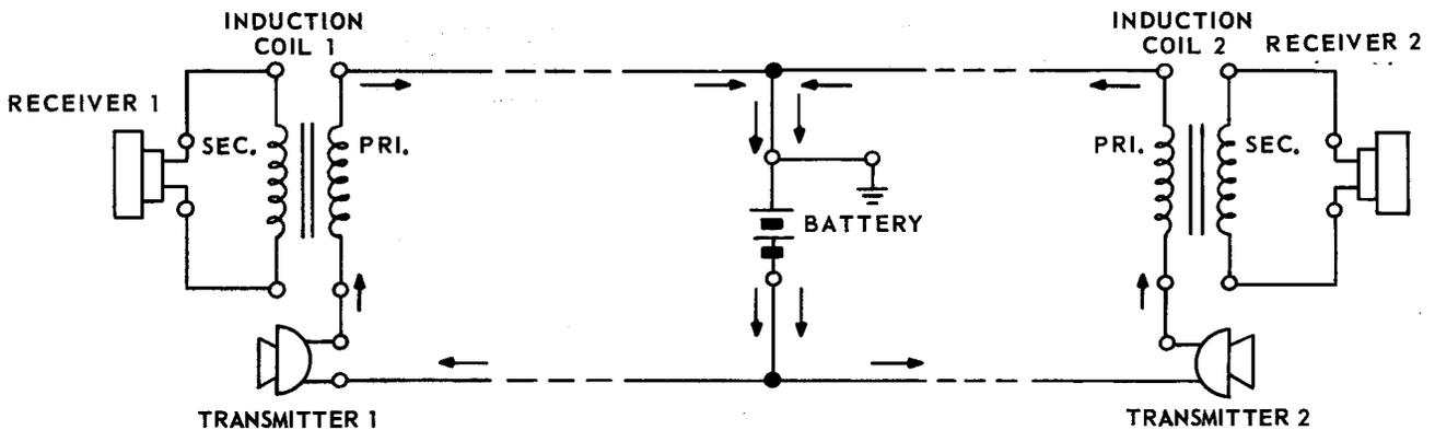
Figure 2-9 Common Battery Telephone System
