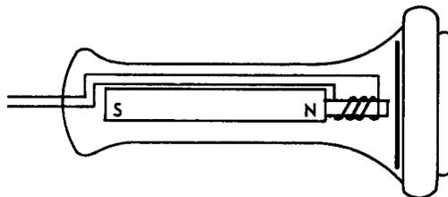
Figure 2-2 Bar-Magnet Transmitter-Receiver
