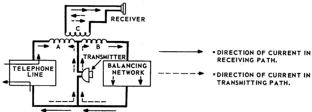
Figure 2-10 Antisidetone Station Circuit
