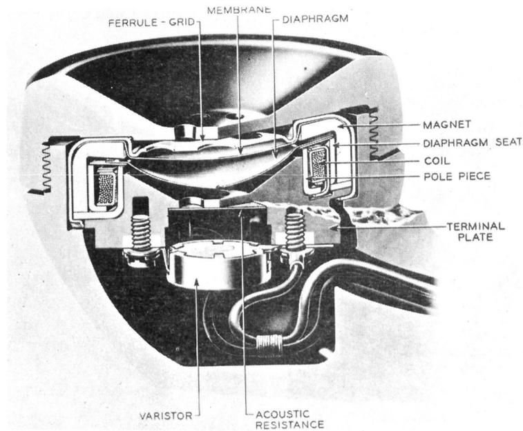
Figure 2-7 Ring-Armature Receiver
