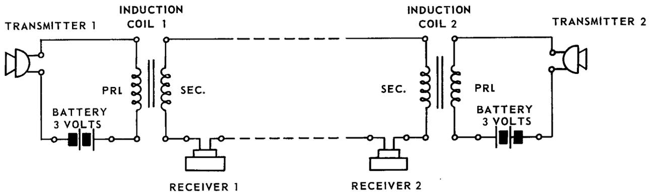
Figure 2-8 Local Battery Telephone Circuit
