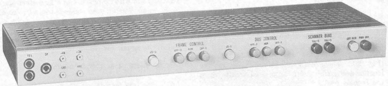
Fig. 14—Scanner Control Panel Using Type 1 through 5 Ferrods
