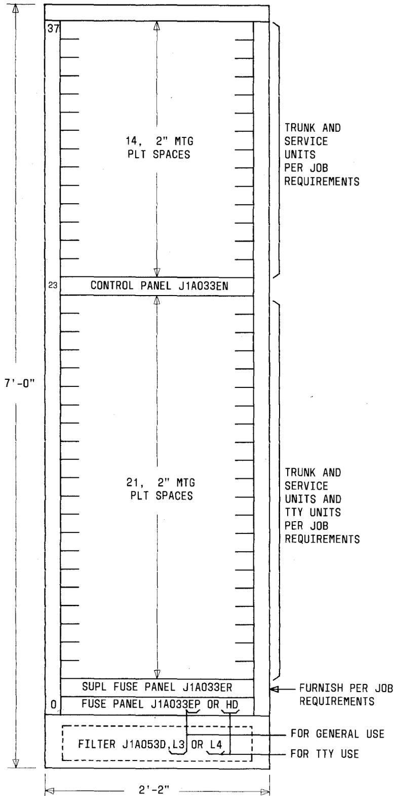
Fig. 5—Miscellaneous Trunk Frame
