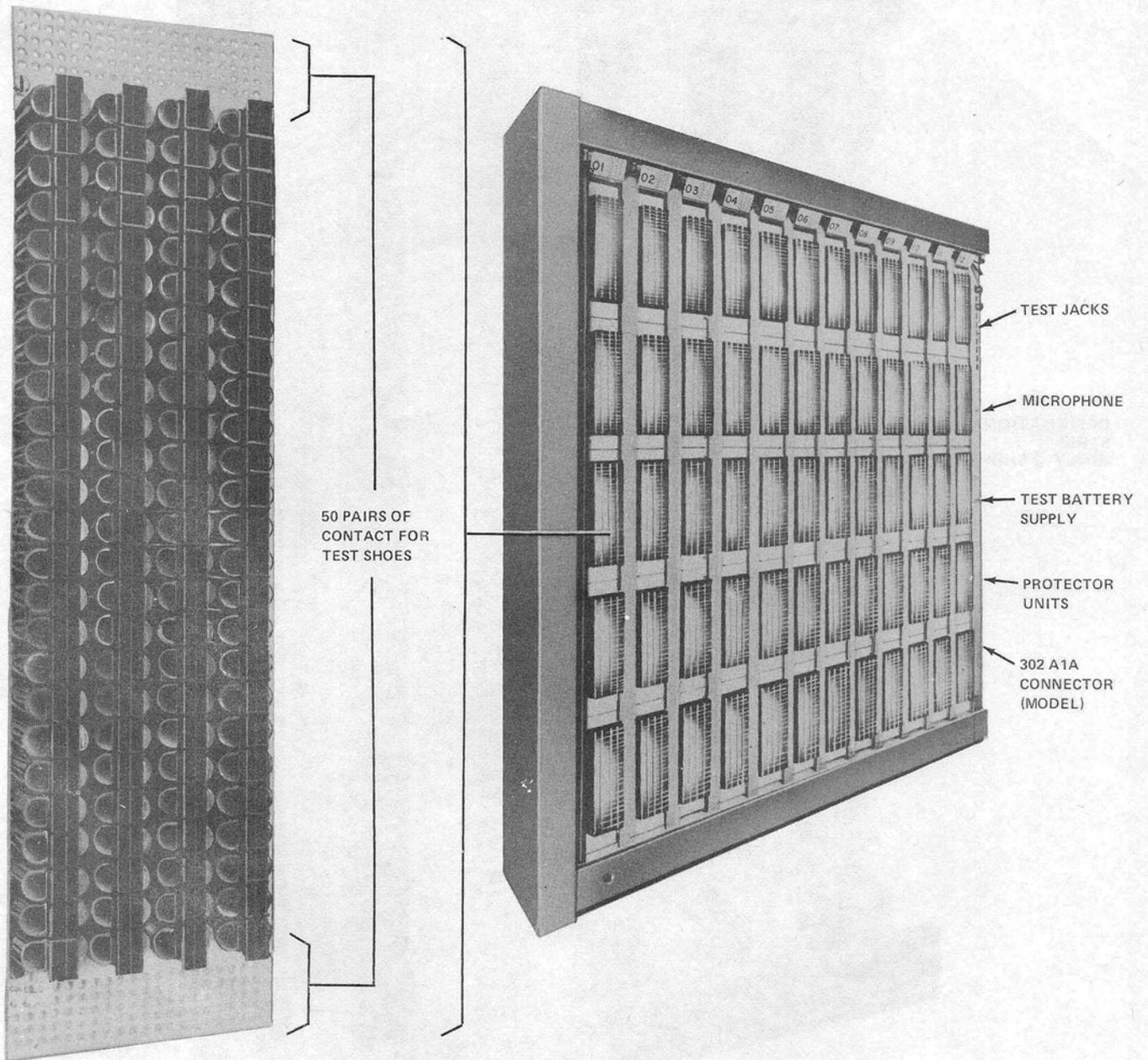
Fig. 2—Protector Frame, Front View
